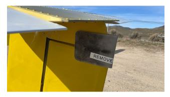
When parked, a metal rudder lock is placed at the top of the rudder and the control stick is secured with the seat belt for the ailerons and elevator.
